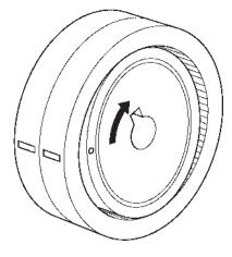
• When the wave generator makes one turn, the flexible gear moves counterclockwise by 2 teeth because the flexible gear has 2 fewer teeth than the stator gear. The driven gear and the flexible gear have the same number of teeth, so their rotational movements are identical. Therefore, the driven gear (output) moves by 2 teeth.
