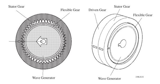
• For example, if the wave generator (input) rotates clockwise while pushing the flexible gear, due to the rotational movement of the DC motor, the meshed area of the flexible gear and the driven gear and stator gear moves in sequence.
