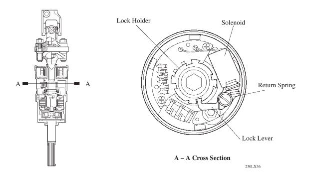
• When the lock mechanism is activated, the VGRS ECU turns OFF the current to the solenoid, and the return spring pushes the lock lever against the lock holder. Then, the lock lever meshes with the groove in the lock holder in order to mechanically lock the movement of the DC motor. When the lock is disengaged, the VGRS ECU turns ON the current to the solenoid, thus disengaging the lock lever and the lock holder and freeing the movement of the DC motor.
